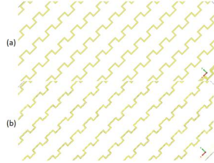
Fig. 5. Fragments of meander-line patterns of the quartz glass within the structure of the linear-to-circular polarization converter (a) drawing on the front-side metallization of the quartz substrate; (b) drawing on the back-side metallization of the quartz substrate
